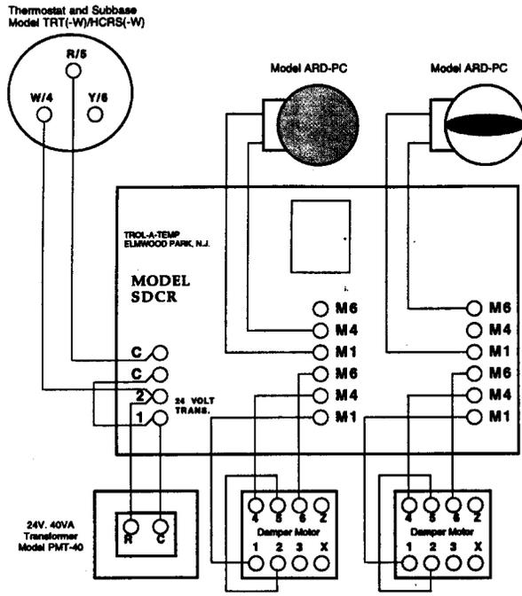
**INTERNAL WIRING DIAGRAM**
